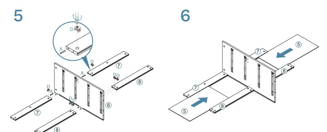
Attach panels [7] and [8] to panel [6] with 2x dowels (A) and secure with 6x locking nuts (D). Tighten with a screwdriver.
