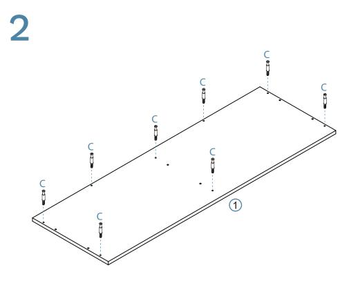
Insert 8x bolts (C) into panel [1] and tighten with a screwdriver.
