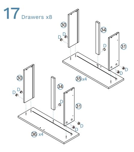
Attach panels [30], [31] and panel [34] to panels [35] and [36] and secure with 40x locking nuts (D). Tighten with a screwdriver.
