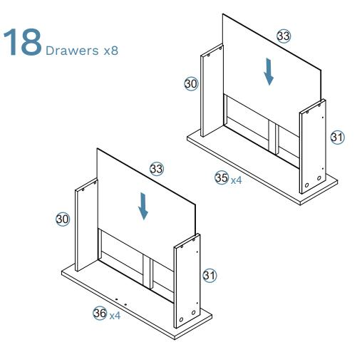
Slide panels [33] down along the grooves between the side panels [30] and [31] as shown.
