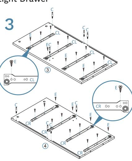
Attach 4x slide rails (CL) to panel [3] and secure with 12x screws (E). Insert 4x bolts (C) into panel [3]. Tighten with a screwdriver. Attach 4x slide rails (CR) to panel [4] and secure with 12x screws (E). Insert 4x bolts (C) into panel [4]. Tighten with a screwdriver.
