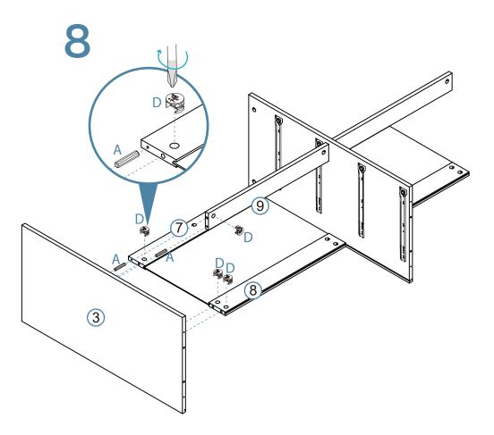
Attach panel [3] to panels [7], [8] and [9] with 2x dowels (A) and secure with 4x locking nuts (D). Tighten with a screwdriver.
