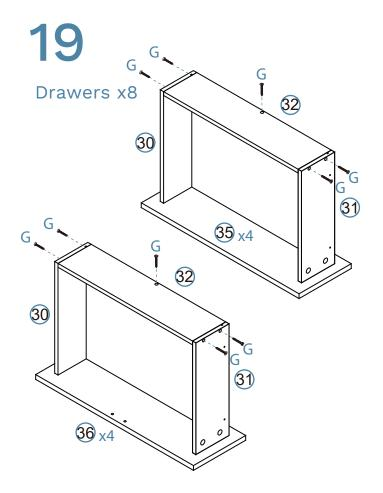
Attach panels [30], [31], [32] and [34] together as shown using 40x screws (G). Tighten with a screwdriver.
