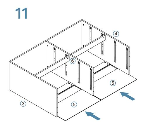
Slide panels [5] down along the grooves between the panels [3], [4] and [6] as shown.
