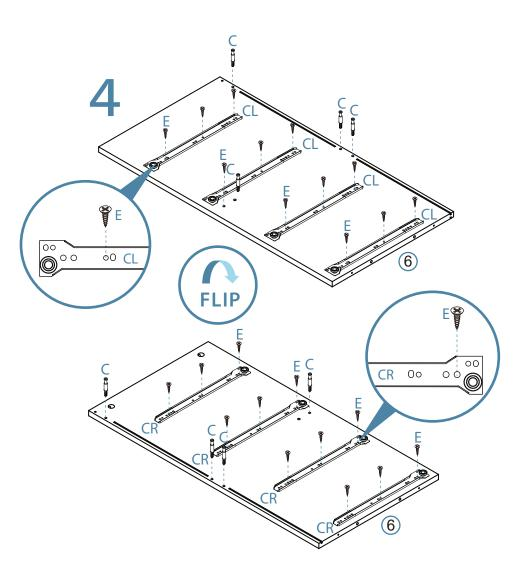
Attach 4x slide rails (CL) and 4x slide rails (CR) to panel [6] as shwon. secure with 24x screws (E). Insert 8x bolts (C) into panels [6]. Tighten with a screwdriver.
