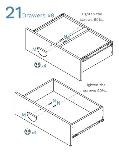
Attach 8x handles (M) to panels [35] and [36] and secure with 16x handle screws (N). Tighten with a screwdriver.
