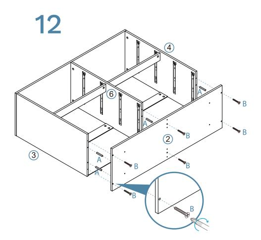
Attach panel [2] to the unit with 6x dowels (A) and secure with 6x screws (B). Tighten with a screwdriver.
