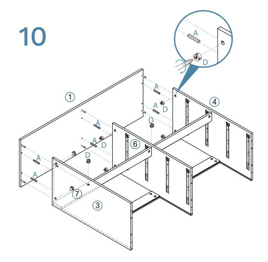
Attach panel [1] to panels [3], [4], [6] and [7] with 6x dowel (A) and secure with 8x locking nuts (D). Tighten with a screwdriver.
