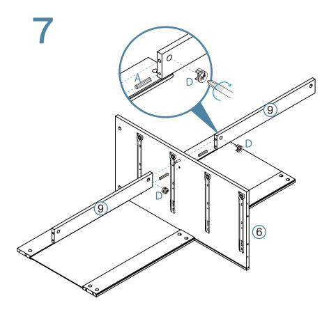
Attach panels [9] to panel [6] with 2x dowels (A) and secure with 2x locking nuts (D). Tighten with a screwdriver.
