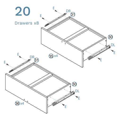
Attach slide rail (DL) and slide rail (DR) to the underside of the side panels [30] and [31] as shown. Secure with 32x screws (E) tighten with a screwdriver.
