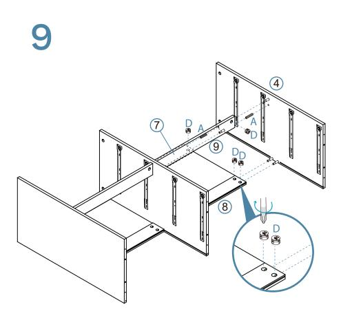
Attach panel [4] to panels [7], [8] and [9] with 2x dowels (A) and secure with 4x locking nuts (D). Tighten with a screwdriver.
